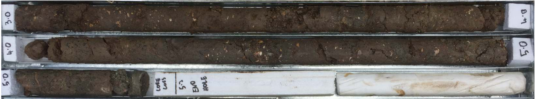
Borehole BH1 – NMLC Core 3.0m to 5.2m
