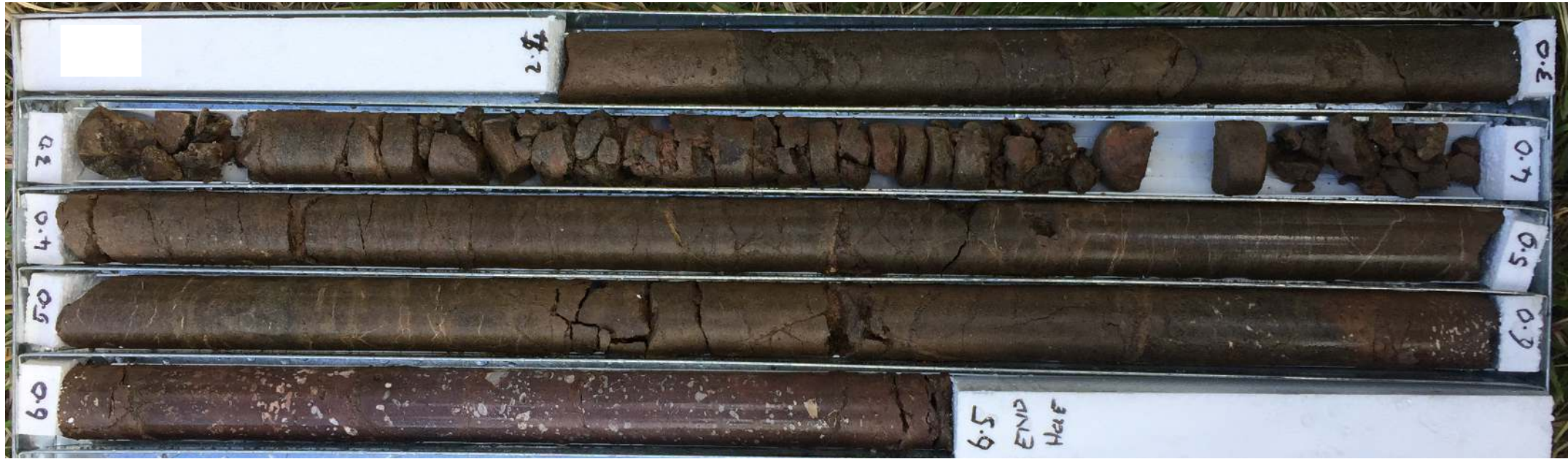
Borehole BH3 – NMLC Core 2.4m to 6.5m
