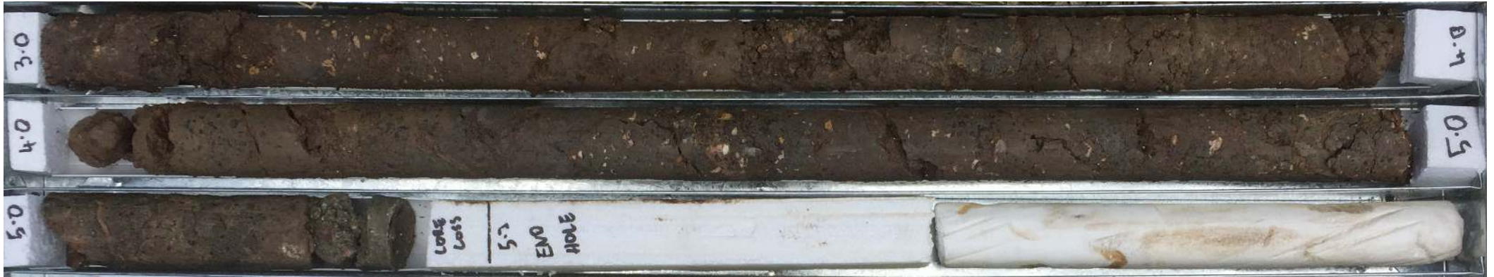
Borehole BH1 – NMLC Core 3.0m to 5.2m
