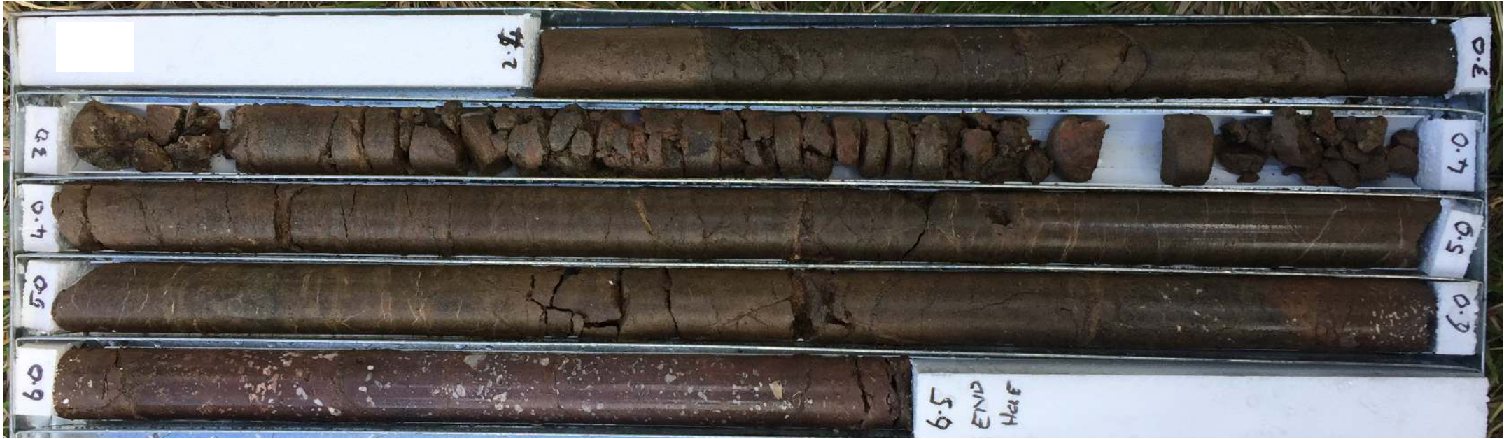
Borehole BH3 – NMLC Core 2.4m to 6.5m
